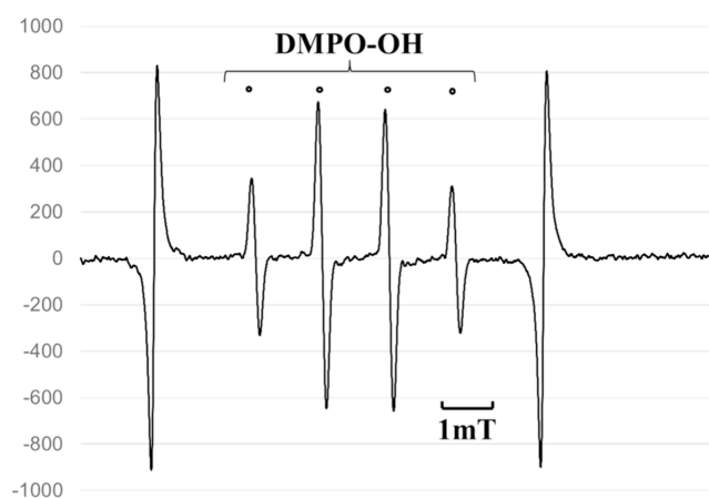
Figure 3. ESR spectrum of the degraded ozone nanobubble water. The spectrum exhibited four distinct peaks with intensity ratios of 1:2:2:1, positioned between those of the Mn 2+ reference standard. The hyperfine splitting constants were A_N = A_H = 14.9 G, indicating the formation of a DMPO–OH adduct.
